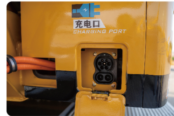
DC charging port
